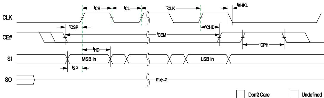
**Figure 19: Input Timing**
