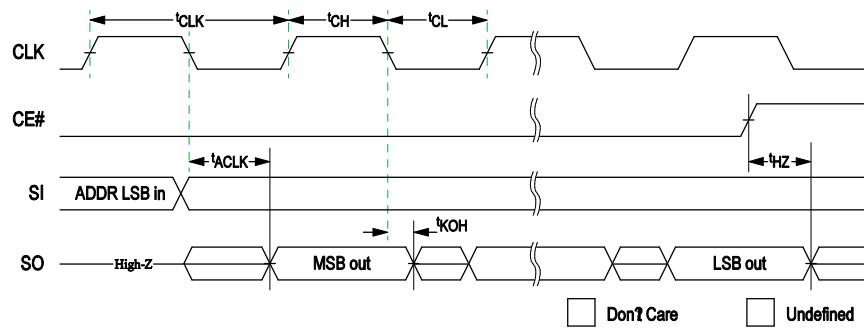
**Figure 20: Output Timing**
