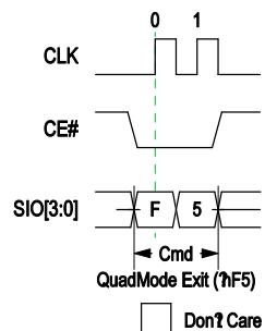
Figure 16: Quad Mode Exit 'hF5 (only available in QPI mode)
