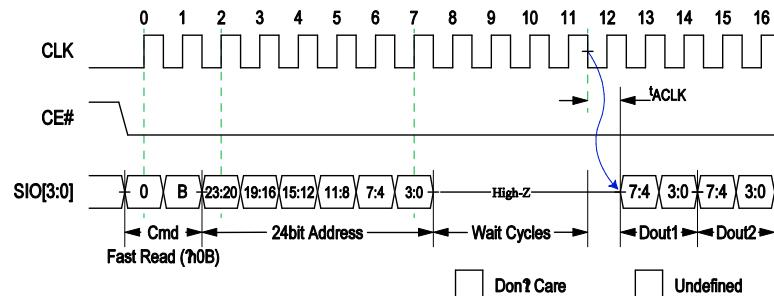
Figure 13: QPI Fast Read 'h0B (max freq 66 MHz)
