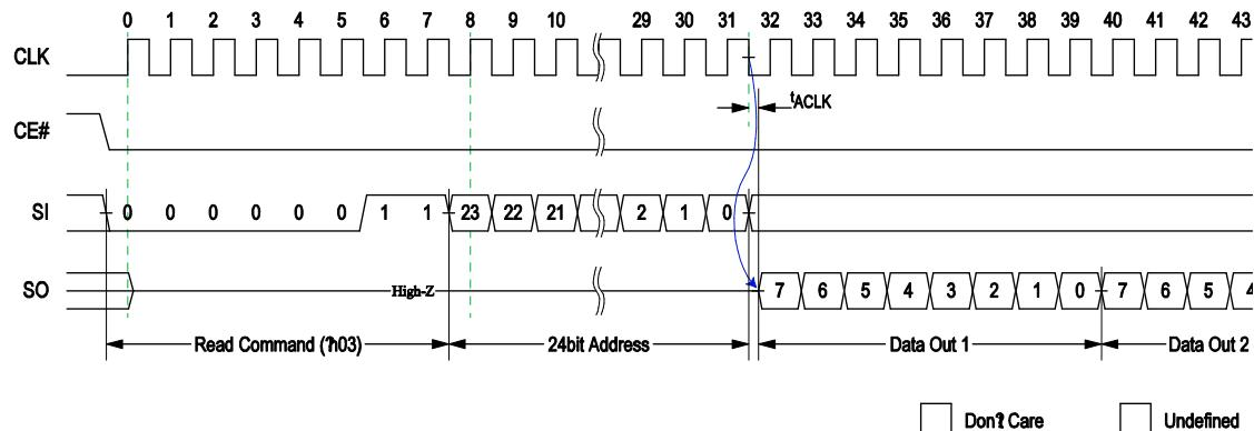
Figure 6: SPI Read 'h03' (max freq 33MHz)
