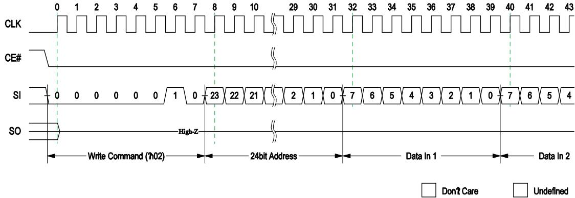
Figure 9: SPI Write 'h02'
