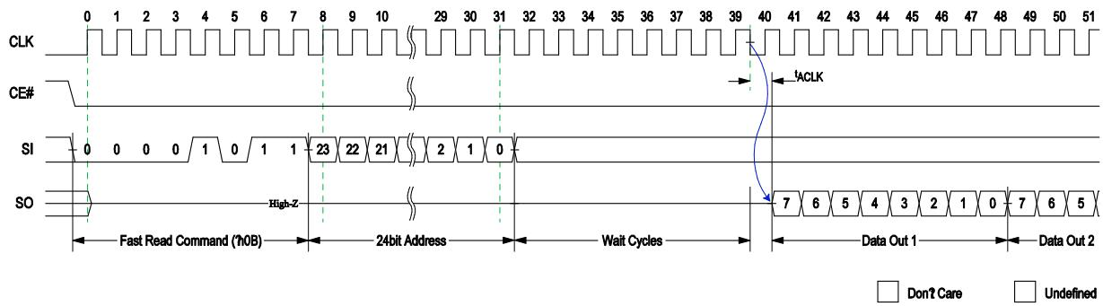
Figure 7: SPI Fast Read 'h0B' (max freq 144 MHz)
